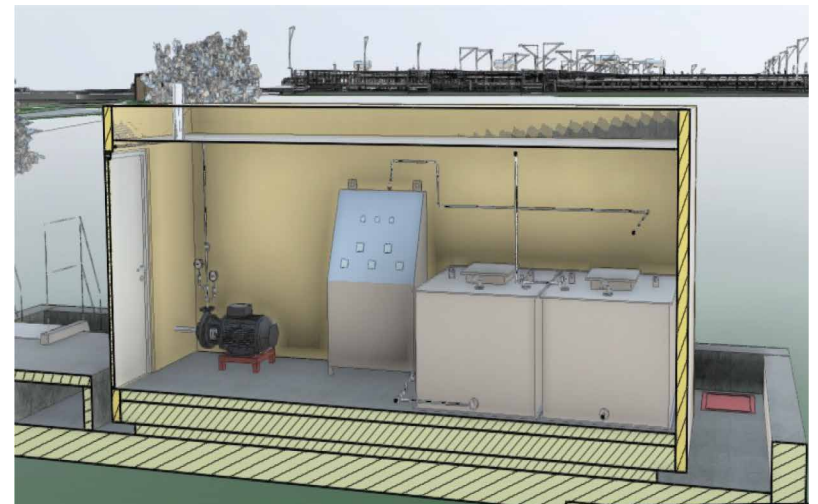
Oxicide dosing station
