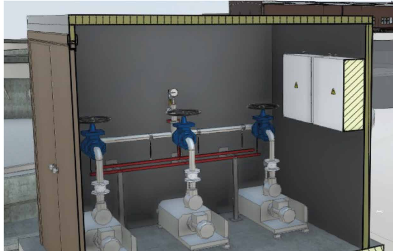
Pumping station for vacuuming
