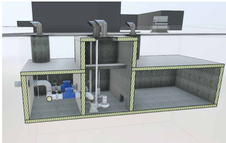
Aerotank emptying pumping station
