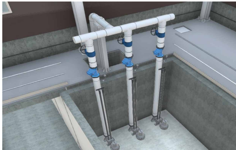
Disc filter building
